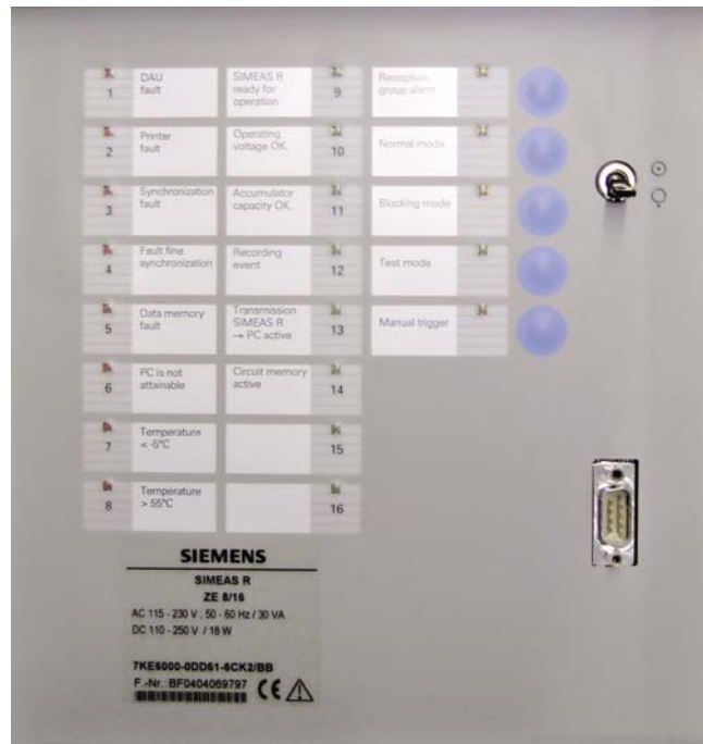
Fig. 13/73 LEDs and control buttons
